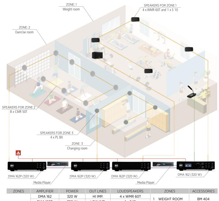
Amplifier output — Audio input — Accessories — 4 channels audio bus — Mute from emergency system
